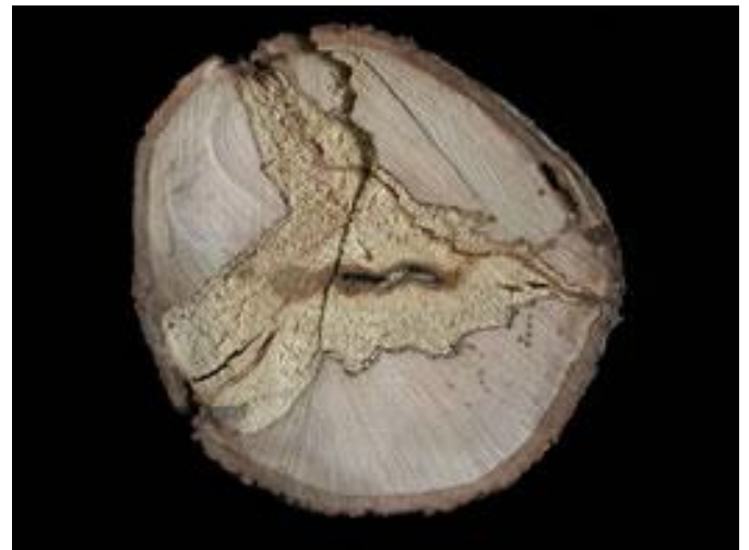
Cross Section Showing White Rot Decay
