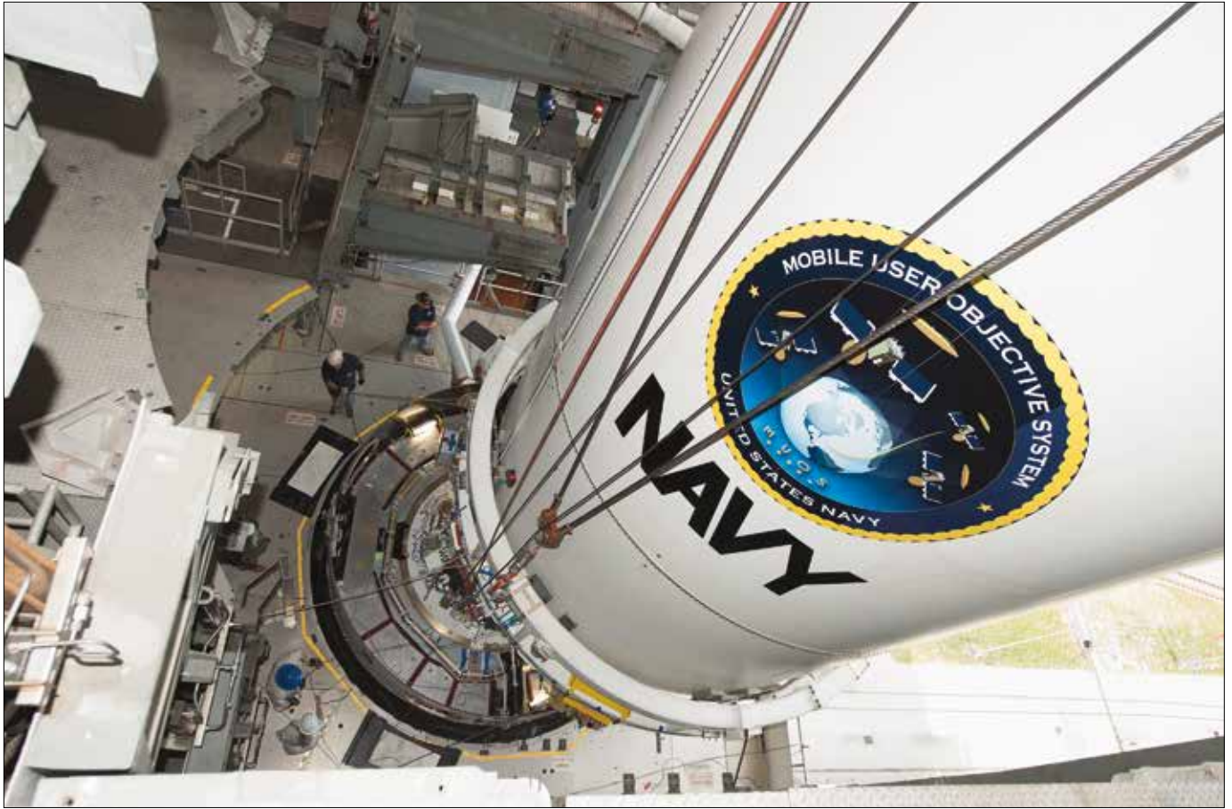
Navy's fourth Mobile User Objective System satellite, encapsulated in 5m payload fairing, stands mated to Atlas V booster inside Vertical Integration Facility at Cape Canaveral's Space Launch Complex-41, August 19, 2015 (Courtesy United Launch Alliance)
