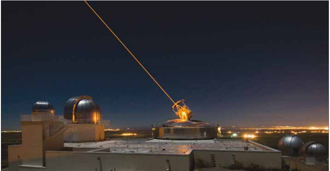
Sodium Guidestar at Air Force Research Laboratory Directed Energy Directorate's Starfire Optical Range provides real-time, high-fidelity tracking and imaging of satellites too faint for conventional adaptive optical imaging systems, November 17, 2005 (DOD)
