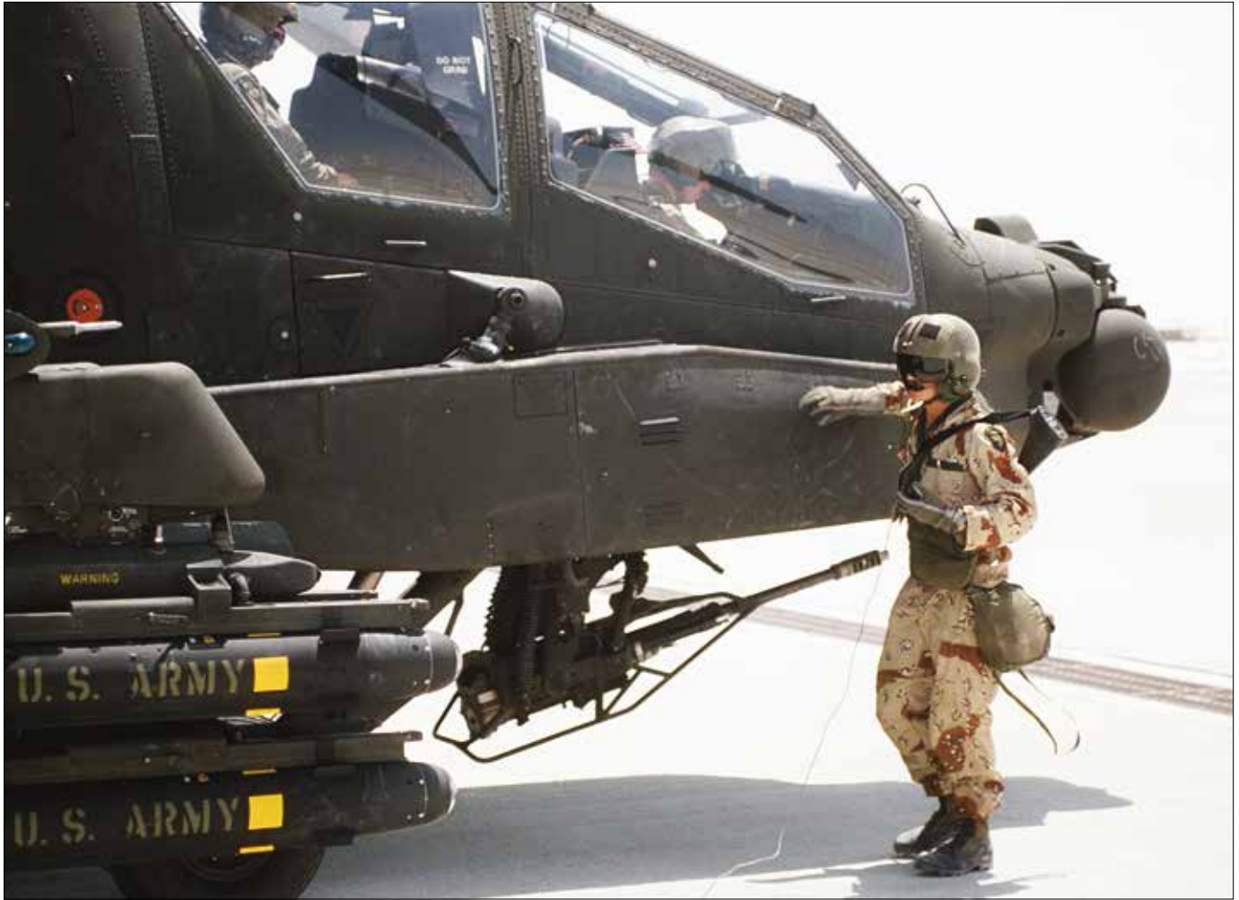
Crewman from 101 st Airborne Division (Air Assault) stands beside AH-64A Apache helicopter armed with M-230A1 30mm automatic cannon and AGM-114 Hellfire missiles as it prepares for takeoff during Operation Desert Shield , January 23, 1991 (DOD)
