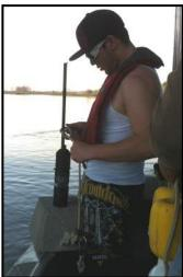
Bill Mole, getting ready to deploy a Test 1 anchor with acoustic receiver attached. The receiver needs greater than 1 meter of water depth to work properly.
