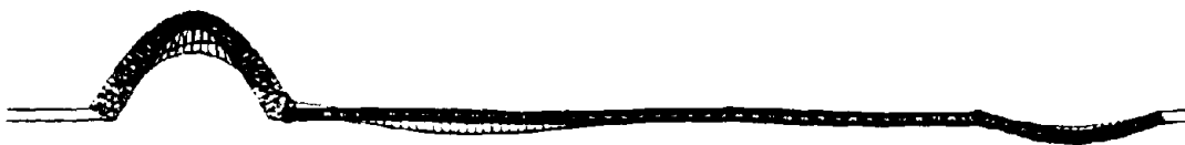
d) Transverse Mode. Mode Number 17. Period = 3.5 seconds
