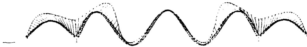
a) Vertical Mode. Mode Number 19. Period = 3.5 seconds
