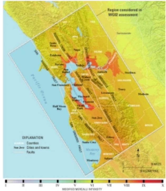
Figure ES.5. Shaking hazard of the SFBR, expressed as the modified Mercalli Intensity (MMI) having even odds of being exceeded in 30 years. Shaking hazard is high throughout the region, and especially pronounced on the soft-soil areas surrounding the bay.
