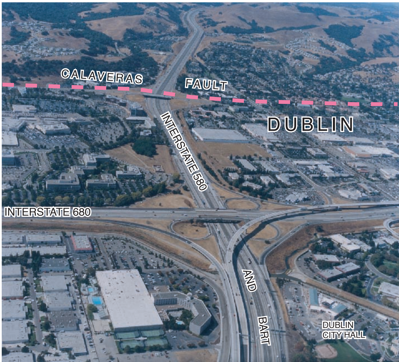
Figure 7.5 Aerial view of the recently (2002) completed Interstate 680-Interstate 580 interchange at Dublin, CA. Note the location of surface trace of the northern Calaveras fault, which crosses I 580 here, and I 680 20 km to the south. All of the high-probability SFBR earthquake sources cross major transportation corridors.
