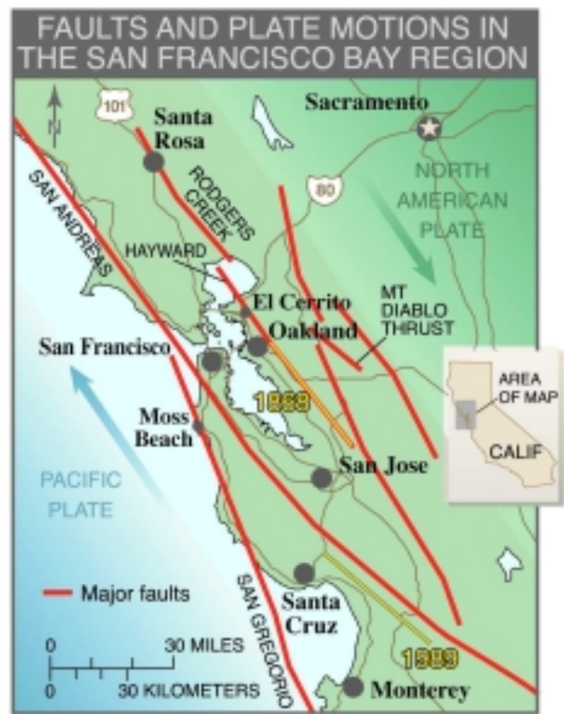
Figure ES.2. Faults and plate motions in the San Francisco Bay Region. Faults in the region, principally the seven faults shown here and characterized in this report, accommodate about 40 mm/yr of mostly strike-slip motion between the Pacific and North American tectonic plates. Yellow lines show the locations of the 1868 M6.8 earthquake on the southern portion of the Hayward Fault and the 1989 M6.9 Loma Prieta earthquake near the San Andreas fault northeast of Monterey Bay.
