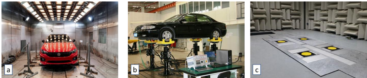
Figure 1. Different applications of single axis road simulators: (a) Tire coupled with climatic chamber, (b) Tire coupled with ambient temperature [7], (c) Tire coupled with acoustic room [9].
