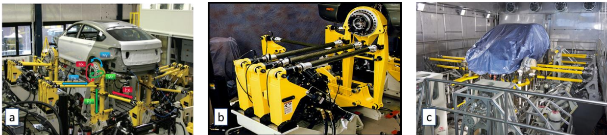
Figure 3. 6 DOF full vehicle road simulation (a) view of the whole system [2], (b) view of the one corner [2], (c) 6 DOF with climatic chamber [5]
