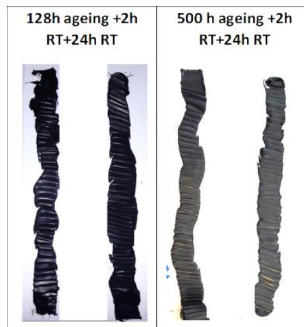
Figure 9: Bead peeled painted metal samples after heat ageing.
