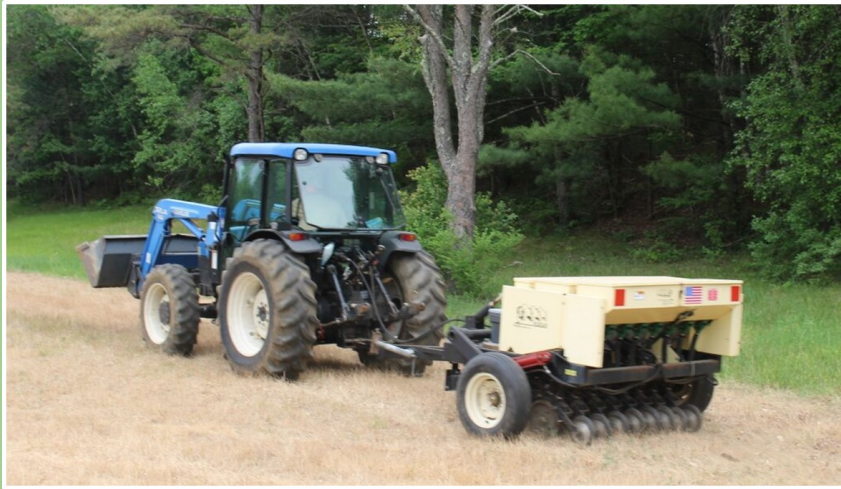
Figure 3.4 Truax no-till drill.
