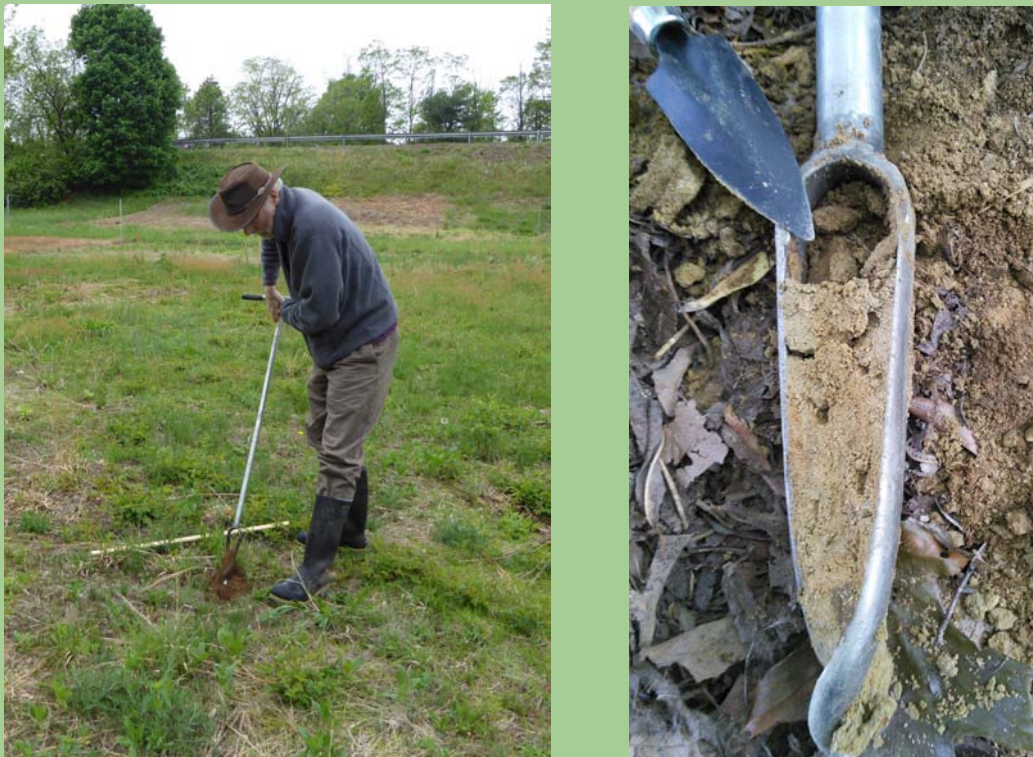
Figure 2.4 Soil scientist Cristian Schulthess conducts redoximorphic feature soil test at site along U. S. Route 6 in Connecticut.
