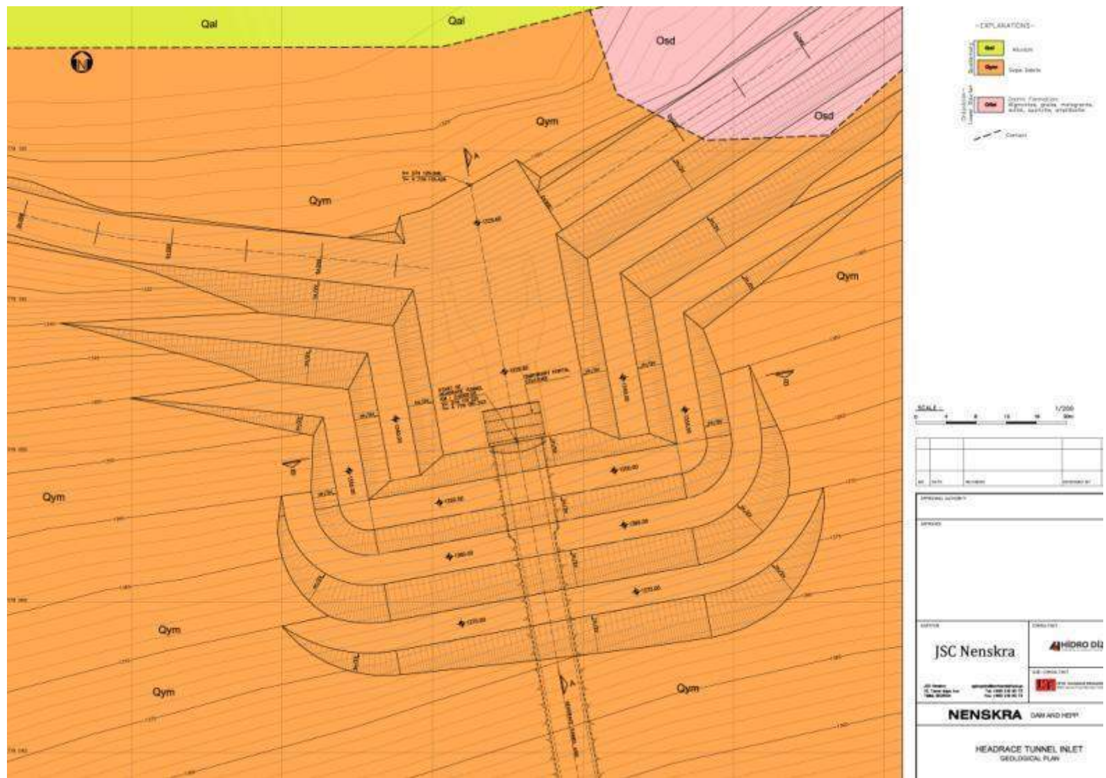
Figure 5.2.3.6.2.3.6. Entrance of headrace tunnel (geological plan)
