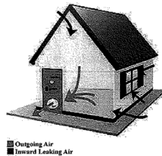
Figure 2. A blower door test measures air leakage and identifies where the home has leaks.
