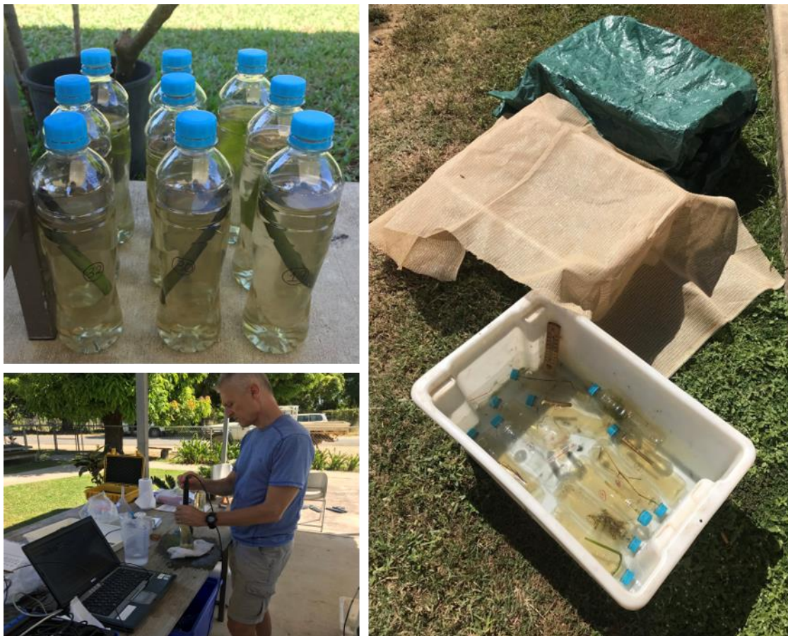
Figure 3-4. Incubation bottles and three light treatments used for measuring algal primary productivity on the Mitchell River floodplain. Photos: Bianca Molinari.
