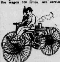
steam can be made in five minutes. steering wheel is provided in front of the seat. The exhaust steam is passed through a feed water heater, and is then delivered to the napths flame, where its presence destroys noise. No skill is needed in the management of the wagon, and it can make ten miles an hour and climb hills with two passongers.—Scientific American.
