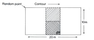
Figure 2: Diagram of the nested quadrat layout used to sample trees  $(20 \times 10m)$ , small trees  $(10 \times 5m)$ , shrubs and herbs  $(5 \times 5m)$ , and ground cover  $(1 \times 1m)$ .
