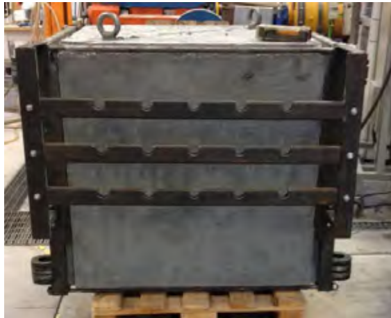
Figure 2 - Strong concrete block, USC ca. 100 MPa. The frame is put on the block and holes are drilled into the block. The diameter of the holes are 46mm and the depth varies between 40 and 50 cm.
