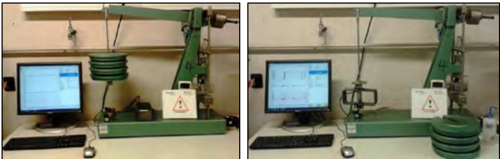
Figure 4. Oedometer setup for the compaction step, left, and the swelling stage, right.
