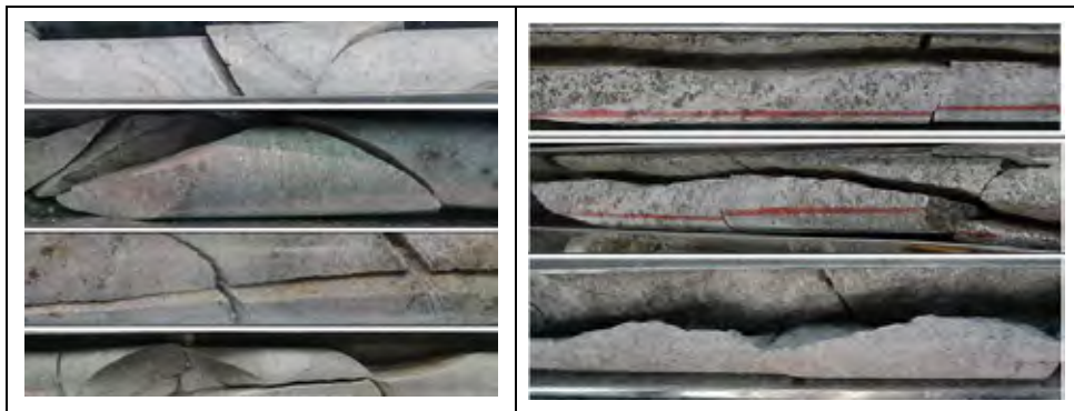
Figure 5 Evaluation of Q -parameters is not an exact science, and there is room for limited differences of opinion. Here are photo-examples of J_r stretching from 1.0 (smooth-planar) to 1.5, 2.0 (smooth-undulating), 2.5 and even 3.5 (extremely rough-undulating). There is no 'law' against using J_r > 3 .
