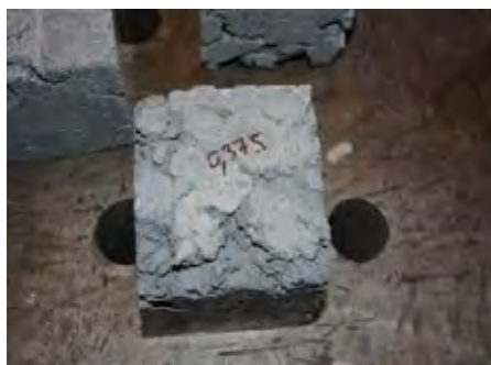
Figure 6 – Grout was too thick and dry.
