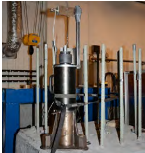
Figure 4 – The length of the bolts from the top of the concrete block up to the end of the bolts is the same for every bolt or 75 cm. The stretch length of the bolt (the length of the base and the cylinder) is however, 60 cm.
