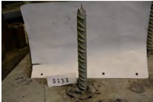
Figure 11 – 40 cm embedment length. The embedment length was longer than the critical length, so the bolt broke. The reduction in diameter closest to the breakage increased until the bolt broke. The maximum load reached 200 kN.
