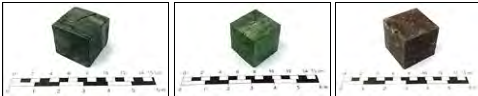
Figure 9: Photos of prepared rock cubes for 3D free swelling, from left to right; alum shale, greenschist and tuff.
