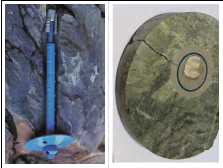
Figure 11 Because single-shell (NMT) relies on high quality S(fr) and long-life rock bolts, the multi-layer corrosion protection methods developed by Ørsta Stål in the mid-nineties, became an important part of NMT. The left photo shows a blue-coloured PVC sleeve: there are also CT-bolts with black, or white, PVC sleeves, as seen in Figure 10. The over-cored CT bolt shown on the right, has a joint/crack deformation next to the bolt (an expected mechanism when installing close to the tunnel face) which does not initiate a potential process of corrosion. Such cracking might lead to the onset of corrosion in the case of a conventional bolt without the PVC sleeve.
