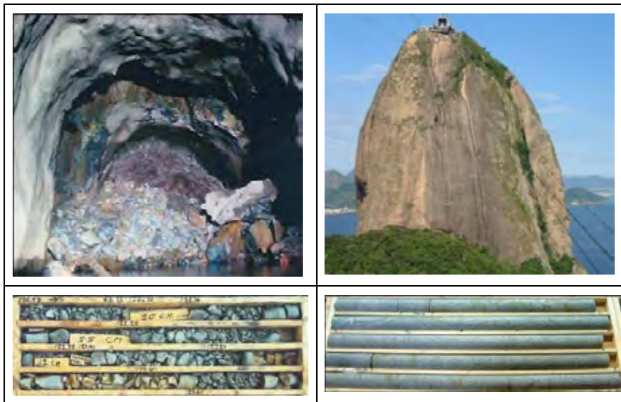
Figure 1 Contrasting worst ( Q \approx 0.001 ) and best ( Q \approx 1000 ) rock mass qualities. Examples from Brazil (2) Sweden and Hong Kong (the latter due to an unrepresentative vertical hole). The core box with core loss is from the wide regional shear zone at Hallandsås, in S.W. Sweden.
