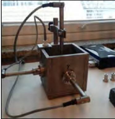
Figure 5: Photo of 3D measuring cell and apparatus for free swelling in 3 directions developed at SINTEF/NTNU in 2013.
