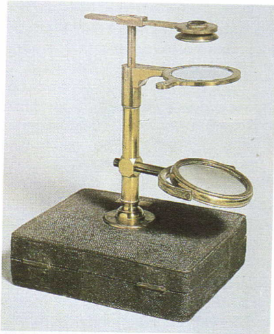
An example of an Ellis aquatic microscope, English, mid-18th century. The instrument dismantles to pack away in its box. (MHS, Oxford.)
