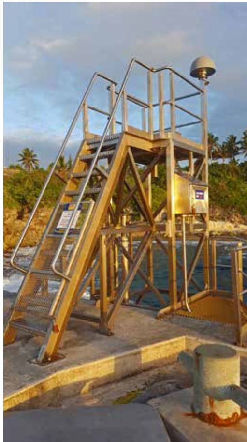
FIGURE 21. Tidal gauge located at Alofi Wharf.
