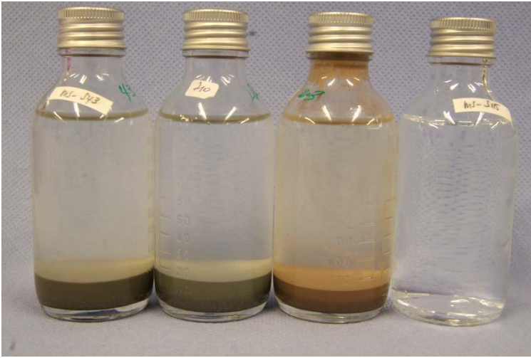
Figure 6. Slurry after water samples taken for \Sigma\text{-CO}_2 . From left to right: DS, WBM, TCC, \text{H}_2\text{O} .
