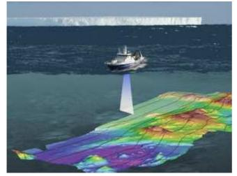
Fig. 5. Diagrammatic representation of the *Tangaroa* multibeaming the seabed of Ross Sea (Image: Erika Mackay, modified John Mitchell).
