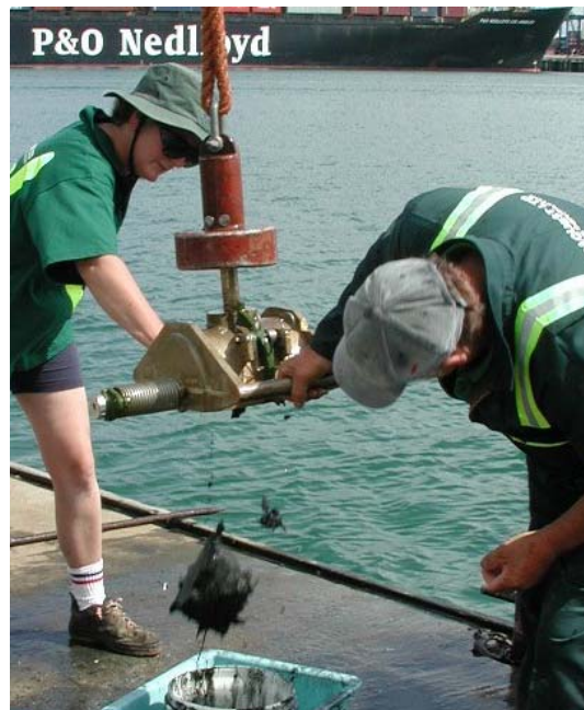
Figure 6: Shipek grab sampler: releasing benthic sample into bucket
