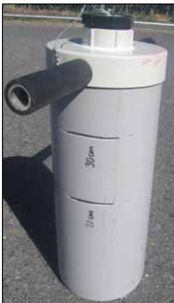
Figure 5: Large hand corer (left) and anchor box dredge (right) for sampling benthic infauna
