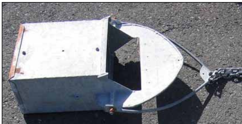
Figure 5: Large hand corer (left) and anchor box dredge (right) for sampling benthic infauna
