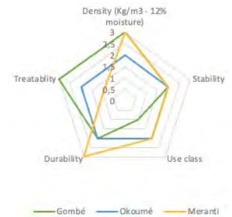
Figure 15 - Technical properties of Kosipo (CIRAD, 2020). Gombé compared with the relevant proxy species Okoumé and Meranti.
