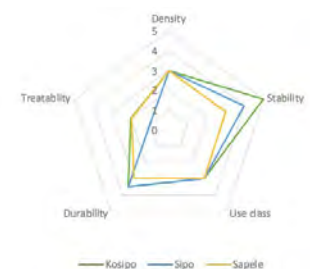
Figure 13 - Technical properties of Kosipo (CIRAD, 2020). Kosipo compared with the relevant proxy species Sipo and Sapele.
