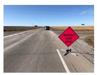
To ensure proper compliance with Federal Highway Administration standards, large fluorescent pink "Emergency Scene Ahead" portable traffic hazard signs are carried in each Patrol Division supervisor's vehicle and in the Crime Scene Investigation vehicle. These signs are to be placed ahead of any traffic-related scene where traffic back-up is anticipated, to provide motorists with proper warning of the incident and to reduce the occurrence of secondary, and sometimes more severe, crashes.
