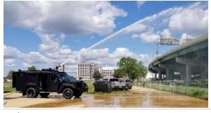
The BearCat is equipped with a roof-mounted nozzle that is hooked directly to a main water line or fire engine for continuous water flow, to enable it to be utilized for fire suppression activities when fire fighters are prohibited from safely accessing a fire scene and tactical deployment is necessary.
