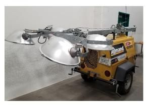
four (4) 1,000-watt metal halide lamps, powerful enough to light an area
