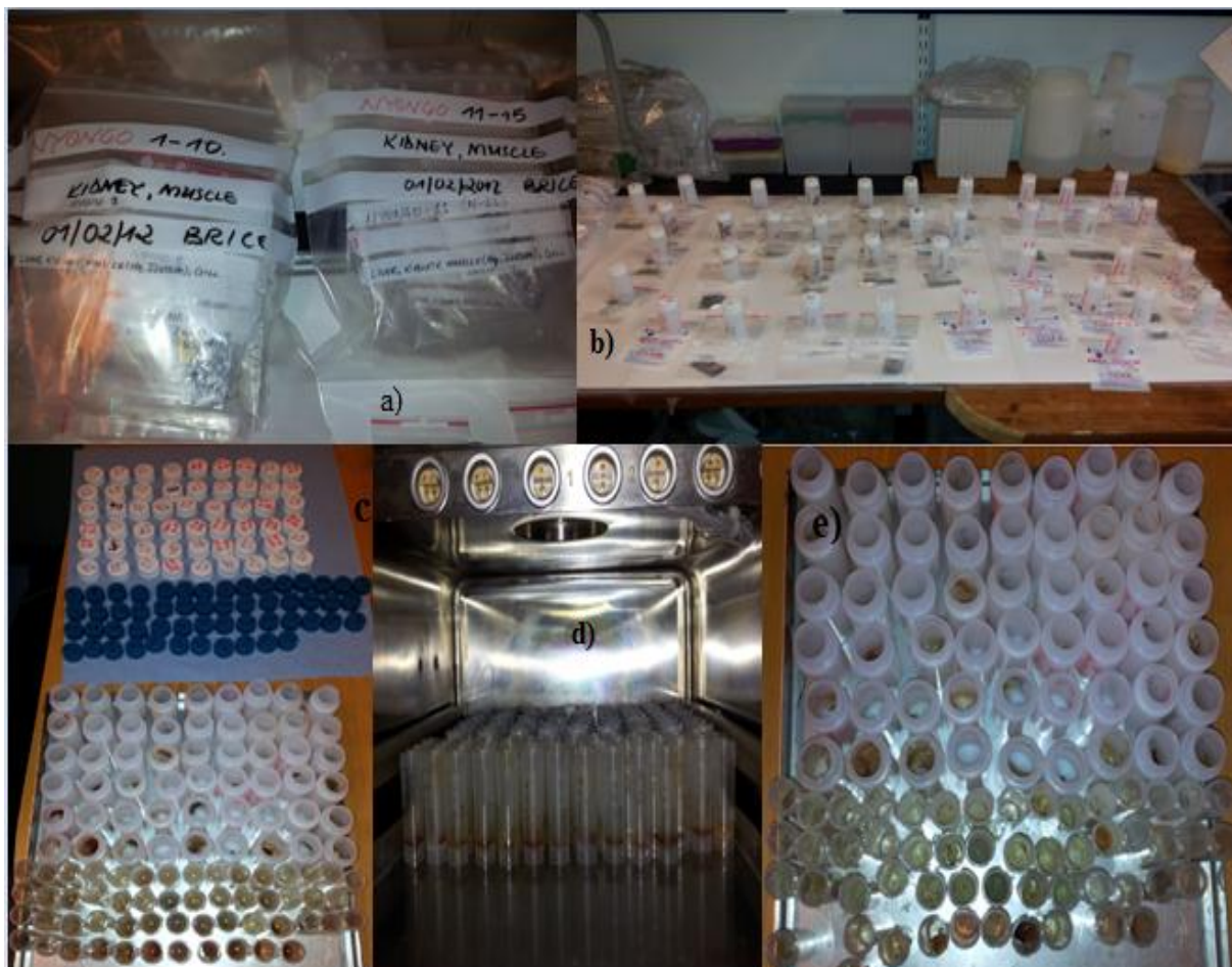
Figure 9. Gill and liver sample handling at IPM laboratory. a) sealed samples, b) sampled tissues sorted with respect to corresponding fish species and codes, c) samples prior to dry freezing, d) samples in freeze drier, e) freeze-dried samples.
