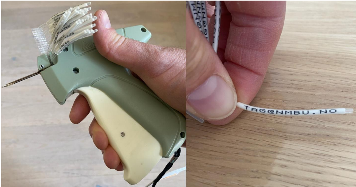
Figure 4. Tagging equipment: Tagging gun (left) and tag bearing a university email address (right)
