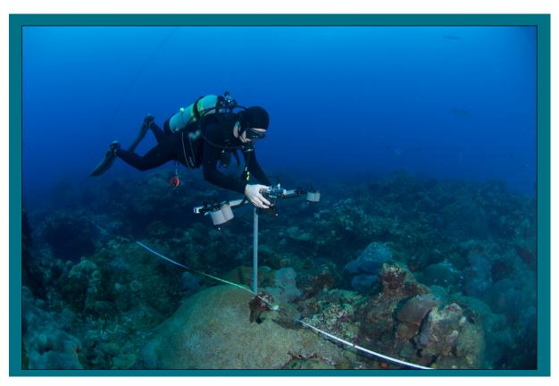
NOAA diver with camera and strobes mounted on an aluminum t-frame takes random transect photographs within the EFGB study site. (Photo: G.P. Schmahl, NOAA/FGBNMS)
