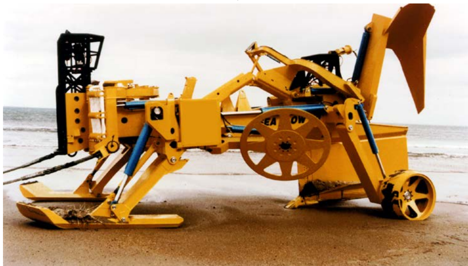
Figure 2: Sea Plow VII, similar to one used for initial PC-1 cable installation across OCNMS. The unit is 8.3 m long, 4 m wide, 4.2 m tall and weighs 14.5 tons.
