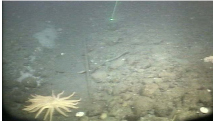
Figure 8. Examples of seafloor disturbance and visible trench along PC-1 cables in OCNMS. Vertical face on side of trench is more distinct in middle photo. Bottom photo shows exposed cable in visible trench through gravel/cobble substrate.
