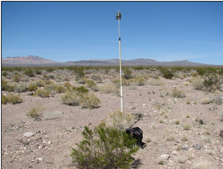
Figure 6-5. Bat detector in a typical Mojave Desert wash north of Little Skull Mountain, Grid Cell 10662.
