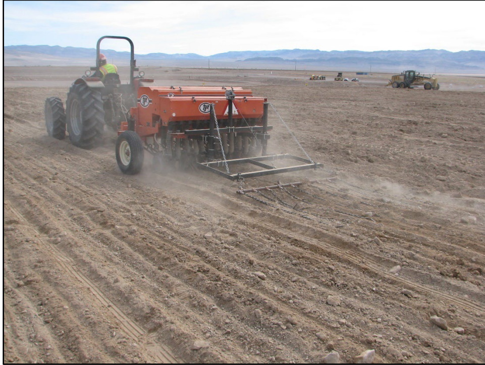
Figure 7-7. Broadcast seeding CAU 577 Cells 19/20 with drill seeder and chain harrow. (Photo taken March 3, 2022, by D.B. Hall)
