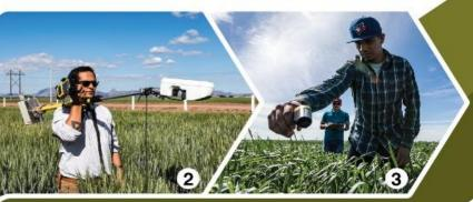
2. Greenseeker for NDVI.3. IR thermometer for canopy temperature.
