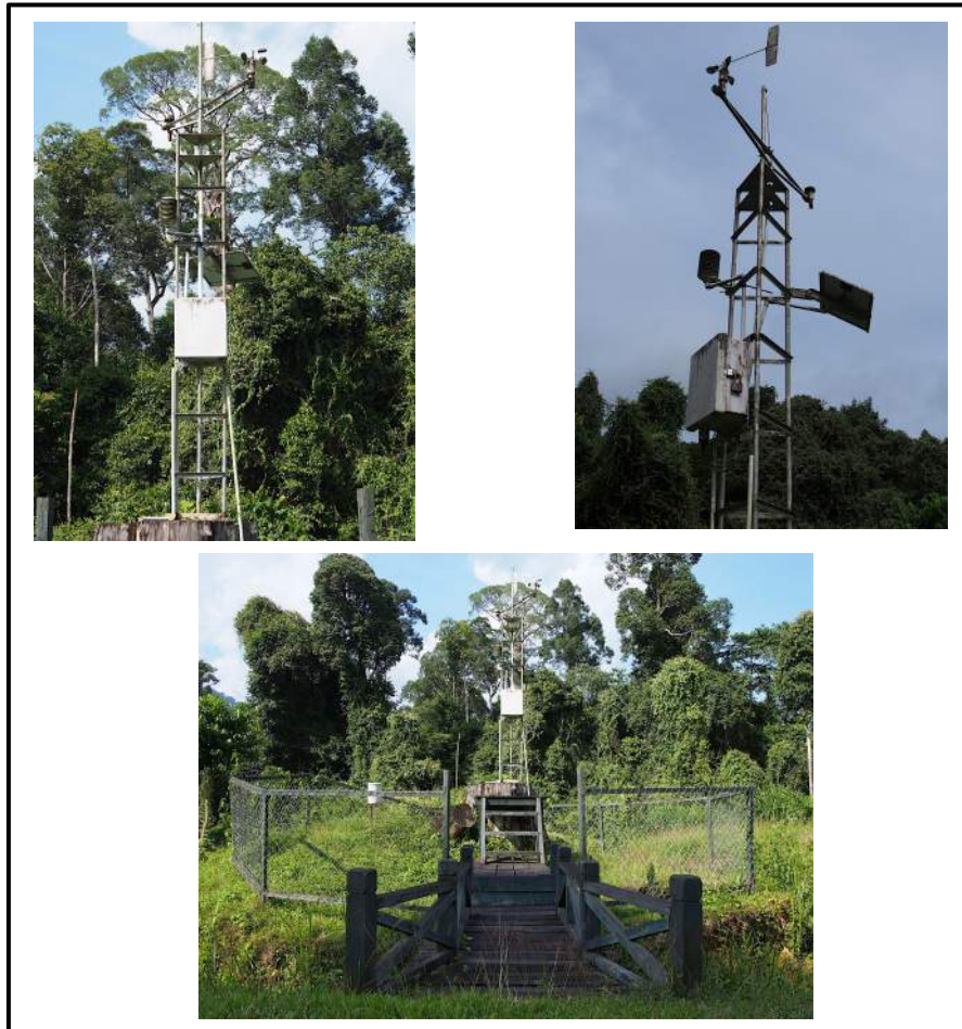
Picture 5.1: Automatic weather Station (AWS) at MBSC
