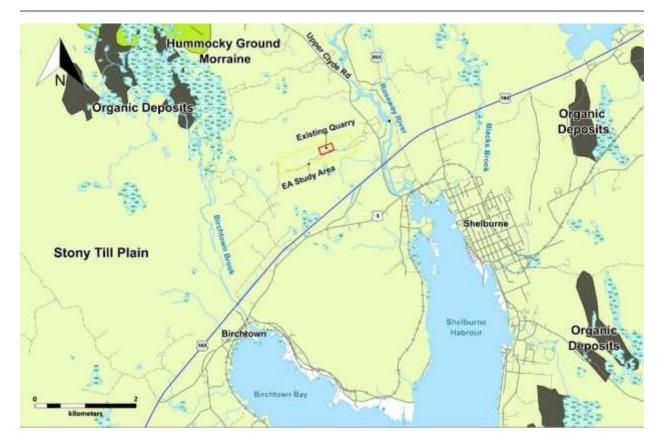
Figure 10. Surficial geology of the study area. From Stea et al. (1992) and digital version (2016).
