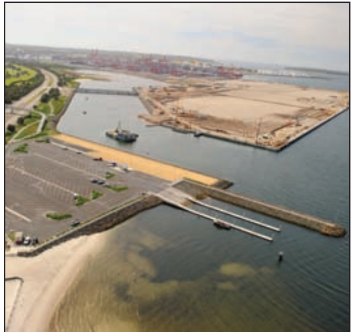
The Port Botany, Australia, extension program was built on 60 hectares (about 148 acres). Applying the Ecosystems Services principle, 1.85 kilometers (about 1.15 miles) of new shipping wharves were brought in balance with habitat enhancement and foreshore beach development for recreation.
