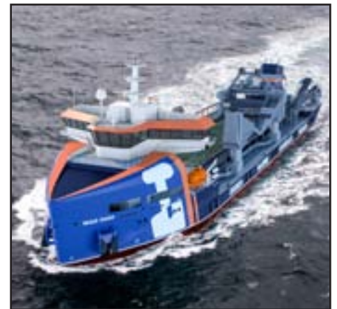
Damen's new trailing suction hopper dredges – Marine Aggregate Dredger (MAD) 4000 and 5600 vessels.
