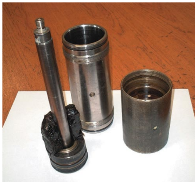
FIGURE 3-18. High-Viscosity Heavy Oil Acquired by Wireline Sampling
