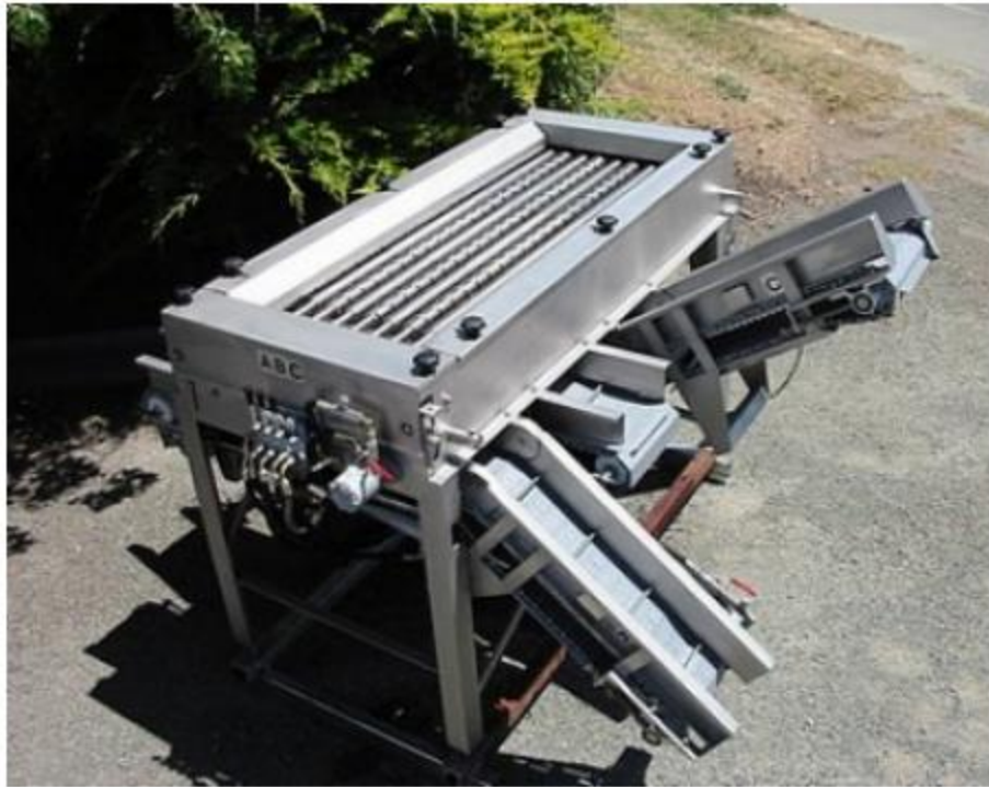
Figure 42. Size grading machine manufactured by Anasco in New Zealand
