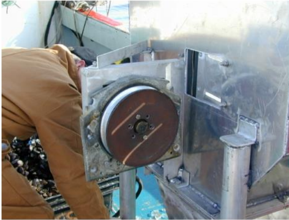
Figure 37. A rear view of the University of New Hampshire's harvesting machine showing the hydraulic hauler. The growing rope is pulled through the slot with stiff rubber flaps to the right of the hauler wheel.
