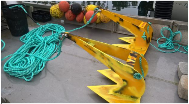
Jeyco Stingray anchors, 75kg, with one-inch co-polymer anchor rode attached.
