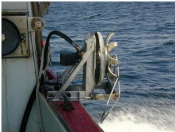
Figure 25. An example of a hydraulically driven starwheel mounted on forward portion the starboard rail of a service vessel. The stainless steel bars on this and in Figure 26 deflect the growing ropes away from the wheel to prevent tangling
