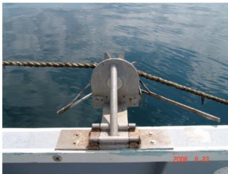
Figure 26. An example of an idler starwheel mounted on the aft portion of the rail of a service vessel.
