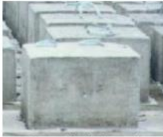
Figure 13: Concrete block with 2 rope loops embedded into the concrete (on top). The rope is tied to the internal rebar supports. Note that the block geometry shown here should not be utilized with this design, as it can be susceptible to tipping.
