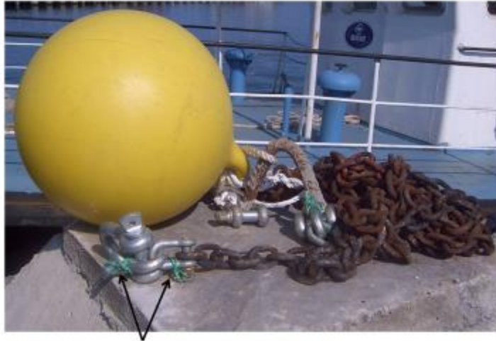
Figure 15: An example of a shackle (shown beneath the yellow float) “moused” with wire to keep the pin from becoming loose during the deployment.
