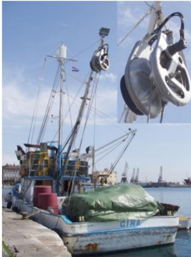
Figure 22. A hydraulic power block on a purse seine vessel. While this equipment is used for another purpose, it may be adapted to raising the backbone if specialized equipment is not available.
