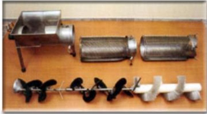
Figure 39. Rubber paddle and brush type declumper manufactured by Talleres Aguin.
