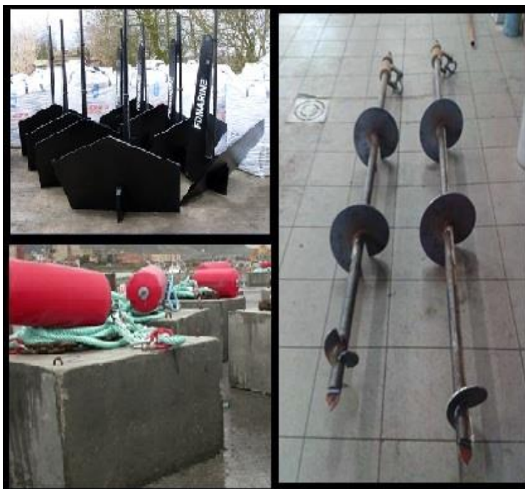
From top left, clockwise: Stingray anchors, helical screw anchors, concrete block anchors. (Photos from Price report (unpublished)).
