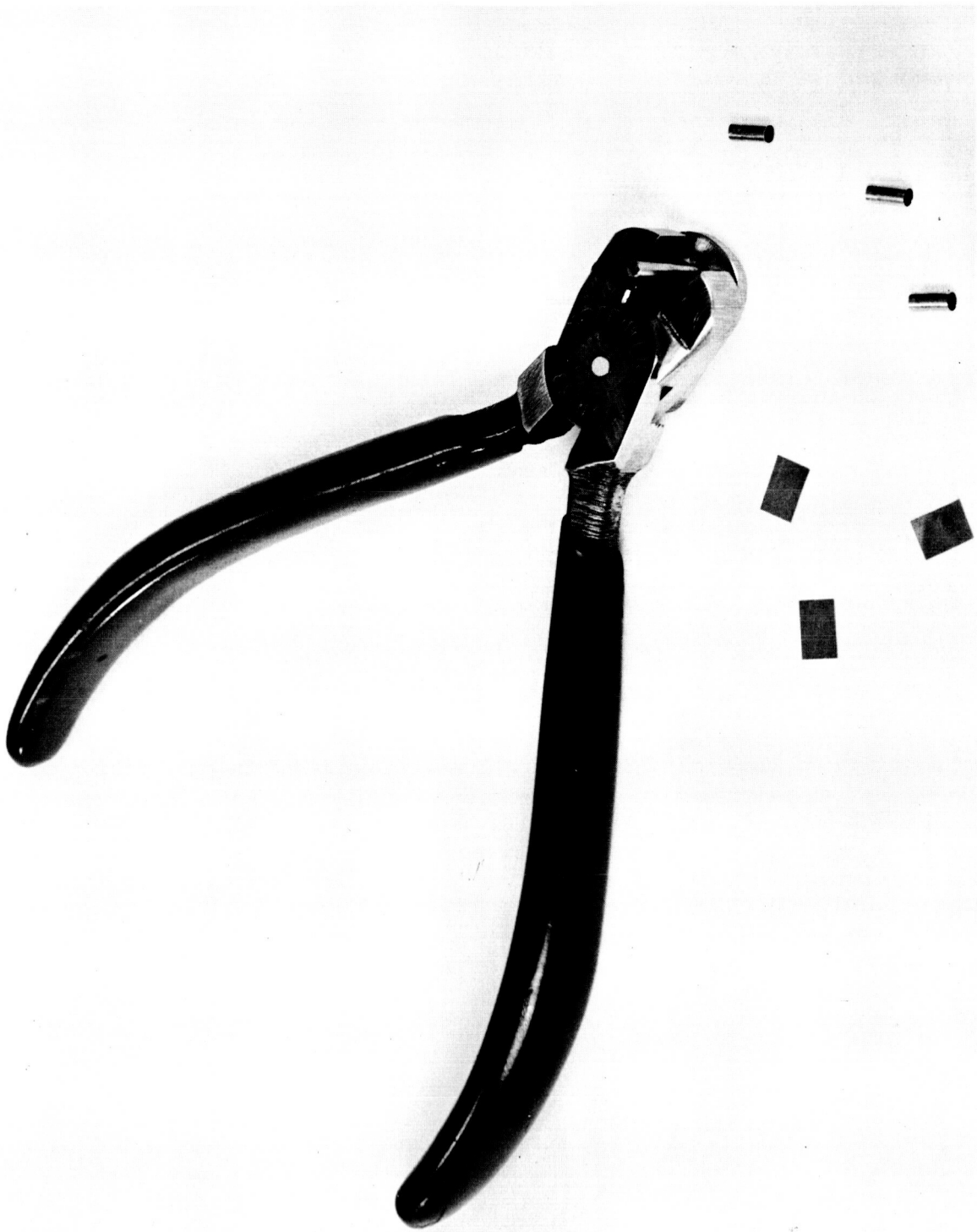
Figure 8. Sleeve-Forming Tool with Flat Stock and Completed Sleeves
