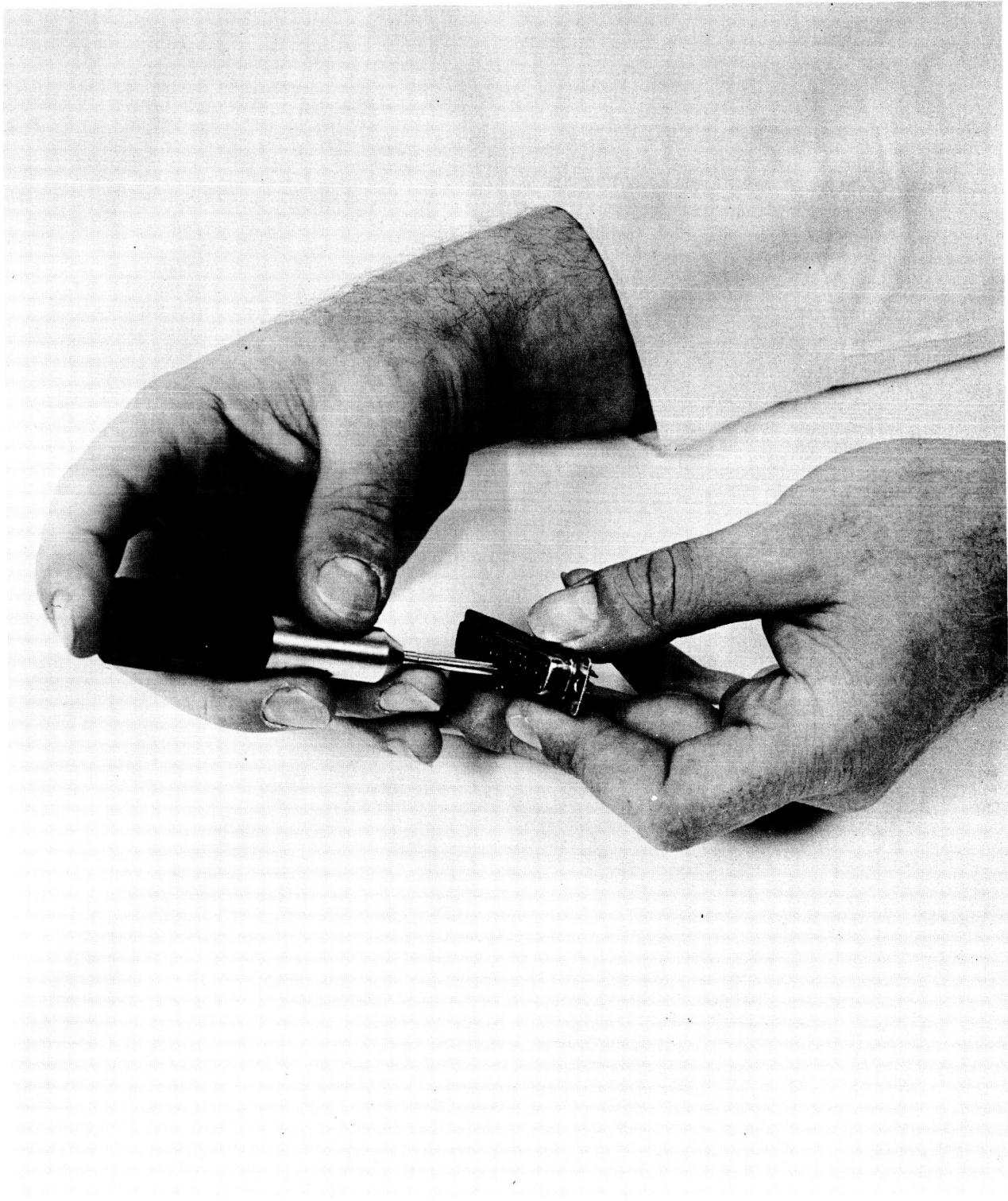
Figure 9. Installing Sleeve on Female Terminal
