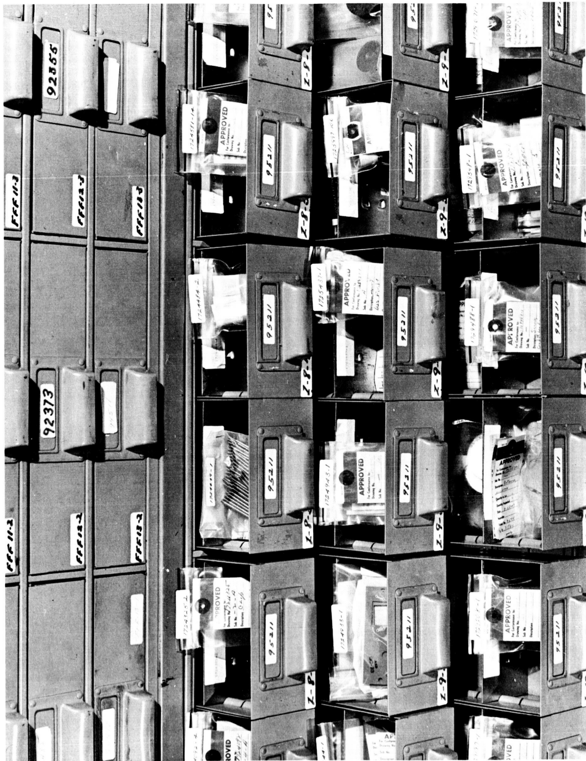
Figure 10. Method of Storing Parts in the Controlled Stores Room
