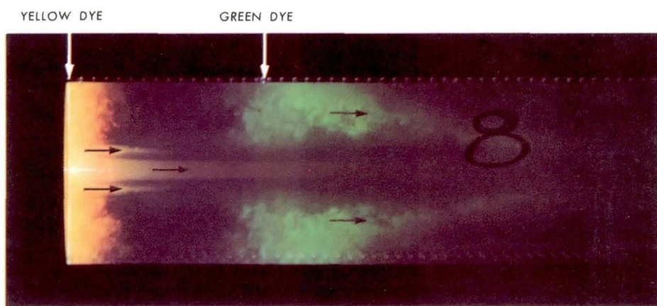
Fig. 10. Dye studies in standard configuration: Views of a portion of the vortex near the closed endwall, at L/D = 6 with nominal \frac{1}{2} -in. exit hole
