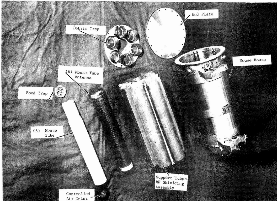
Figure 3 Upper: Assembled prototype hardware designed to study the stability of circadian systems in pocket mice during earth orbital missions (7). Lower: Animal housing assembly disassembled.
