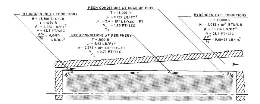
SIDE VIEW OF REFERENCE NUCLEAR LIGHT BULB ENGINE CONFIGURATION
