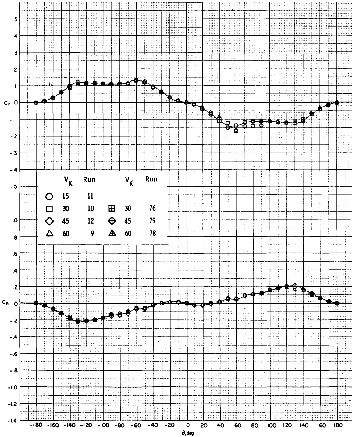
Figure 8.- Effect of windspeed on directional characteristics of model 1 without rotor or tail.
