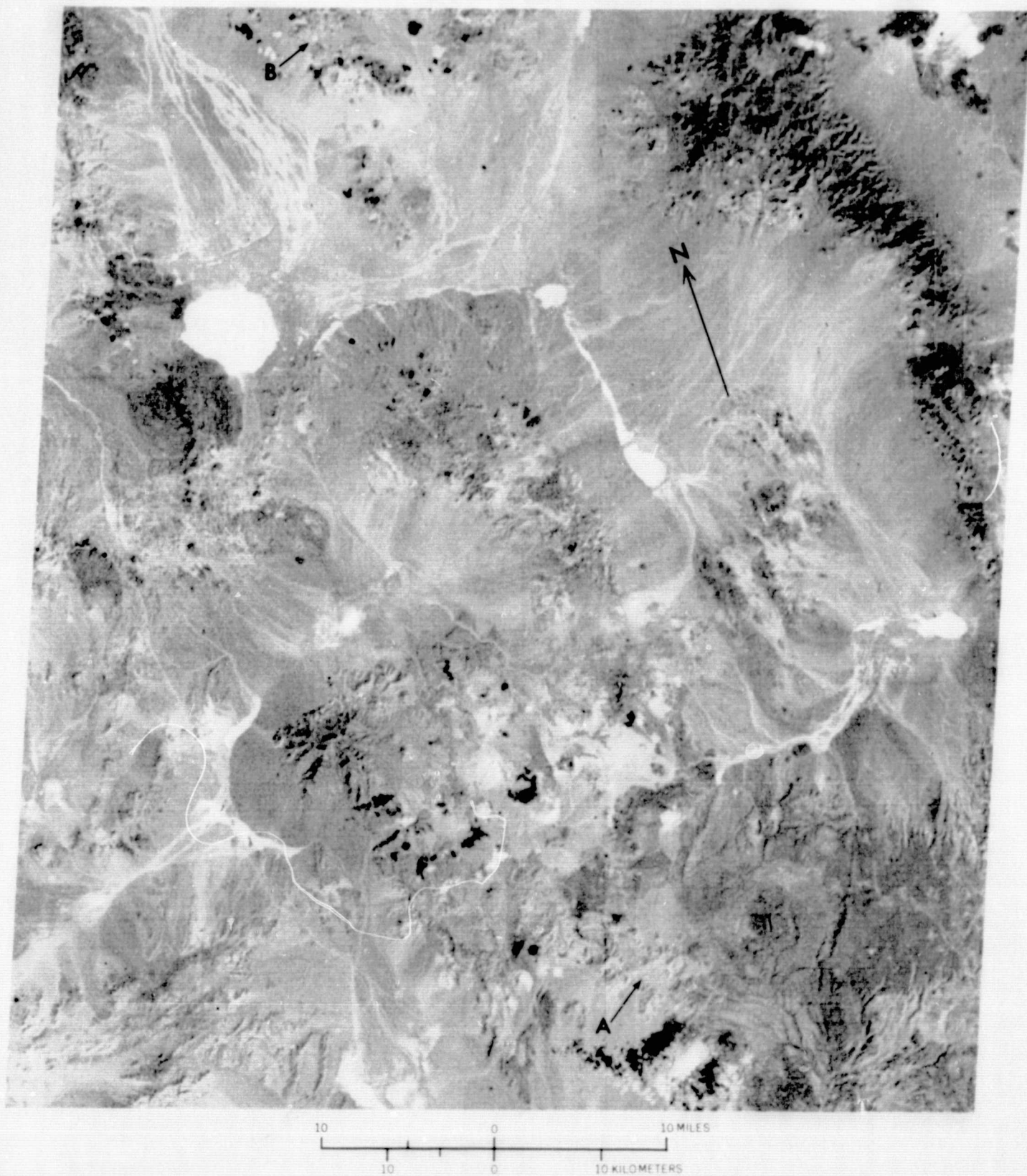
FIGURE 15.—Color-infrared composite of study area made up of linearly stretched images of ERTS MSS bands 4, 5, and 7 with blue, green, and red filters, respectively (scale 1:500,000). A and B are limonitic areas southwest of Quartz Mountain and north of Monitor Peak, respectively. Prepared by the Jet Propulsion Laboratory, Pasadena, Calif., in cooperation with the U.S. Geological Survey.
