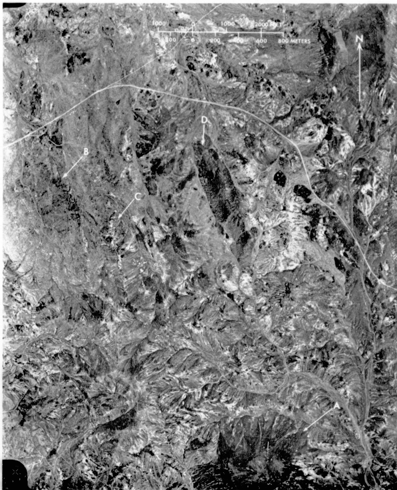
FIGURE 8.—Color aerial photograph of part of the Goldfield mining district: A, unaltered upper Tertiary basalt cap; B, unaltered latite; C, hydrothermally altered andesite and dacite; D, unaltered dacite. Photographed June 2, 1968, for the U.S. Geological Survey. Ektachrome film type 2448.
