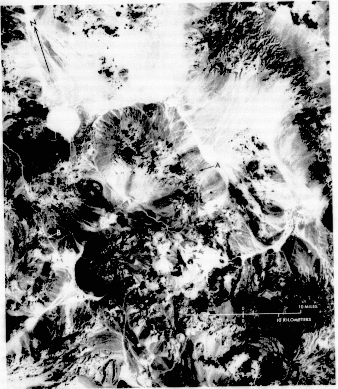
FIGURE 14.—Linearly stretched ERTS MSS image for band 7 of the study area (scale 1:500,000). Note the excellent resolution of the image as evidenced by discrimination of the secondary roads (A) and the main road (B) that passes through Goldfield and south-southeast past Stonewall Mountain. Also note the basalt cap (C) in the Goldfield mining district.
