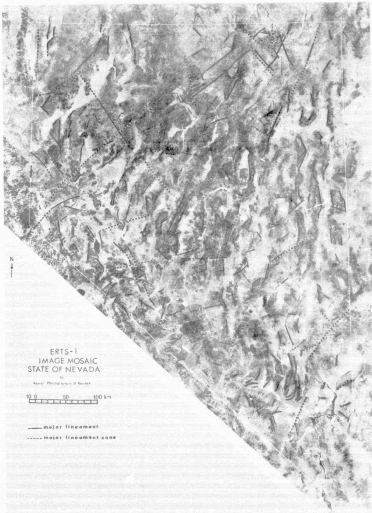
Fig. 3 - Major linear features ( \geq 10 km) plotted on ERTS-1 band 5 image mosaic of Nevada
