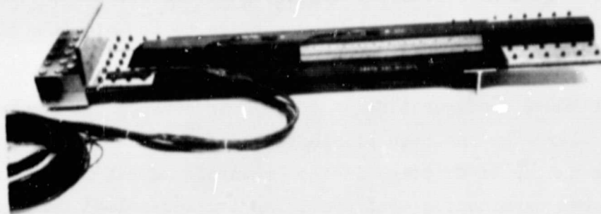
Figure 2-9. Cover to Fuselage Joint Specimen
