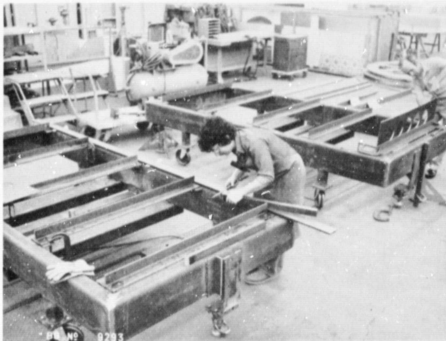
Figure 2-49. Fabrication of Cover Bonding Tools for 100-Inch Subcomponent
