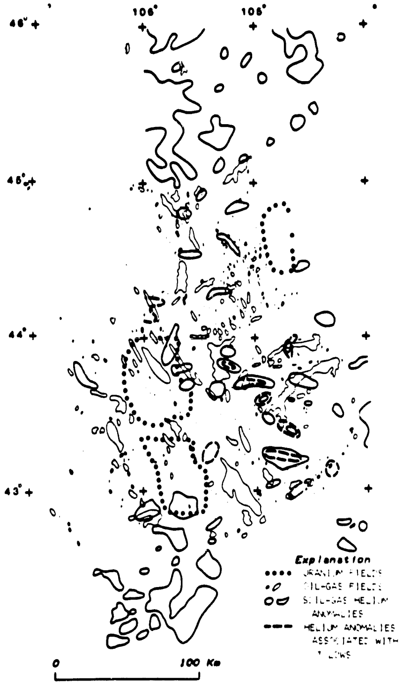
Figure 20.-- Location of helium anomalies, uranium fields, and oil-gas fields in the Powder River Basin, Wyo.
