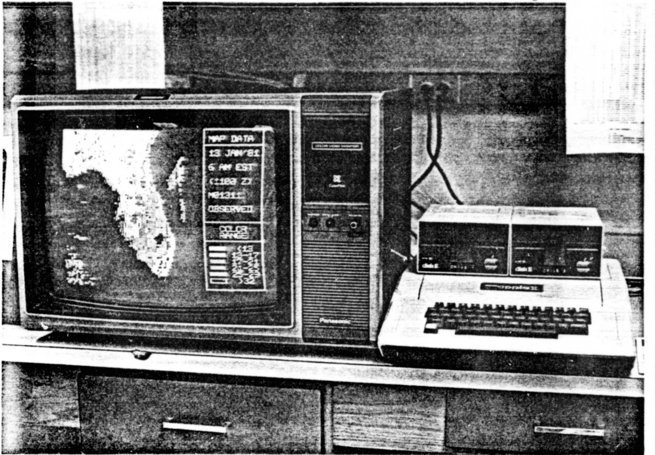
Fig. 7. Apple II Plus used as a SFFS terminal. Two disc drives, a clock, a software controlled modem, and a color monitor are needed for a complete system capable of automatic data acquisition, display and archival.
