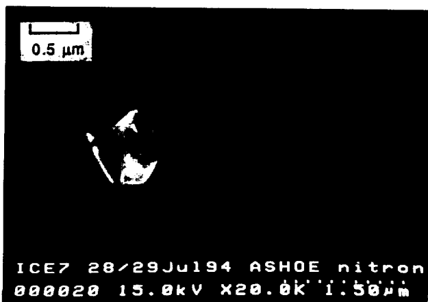
Fig. 1. Ice crystal with nitron-nitrate reaction: Airborne Southern Hemisphere Ozone Experiment (ASHOE) (28 July 1994).
