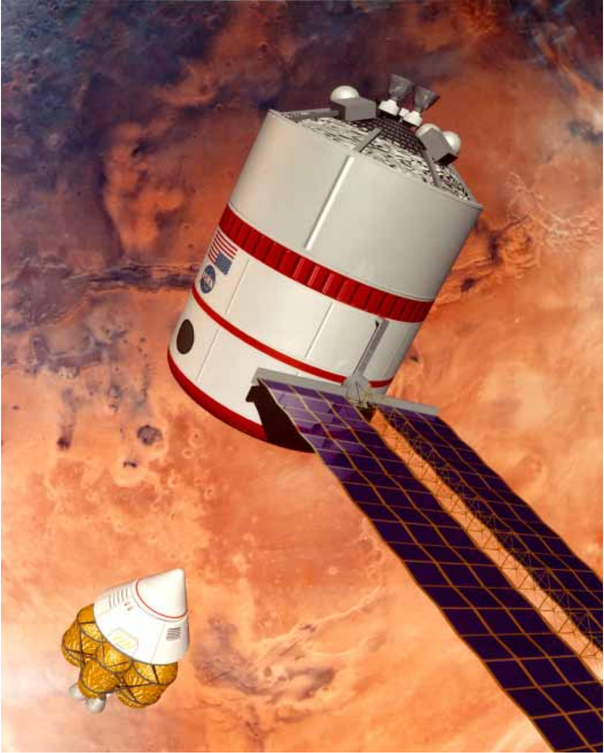
Figure 3-33 Solar array power source for interplanetary spacecraft.
