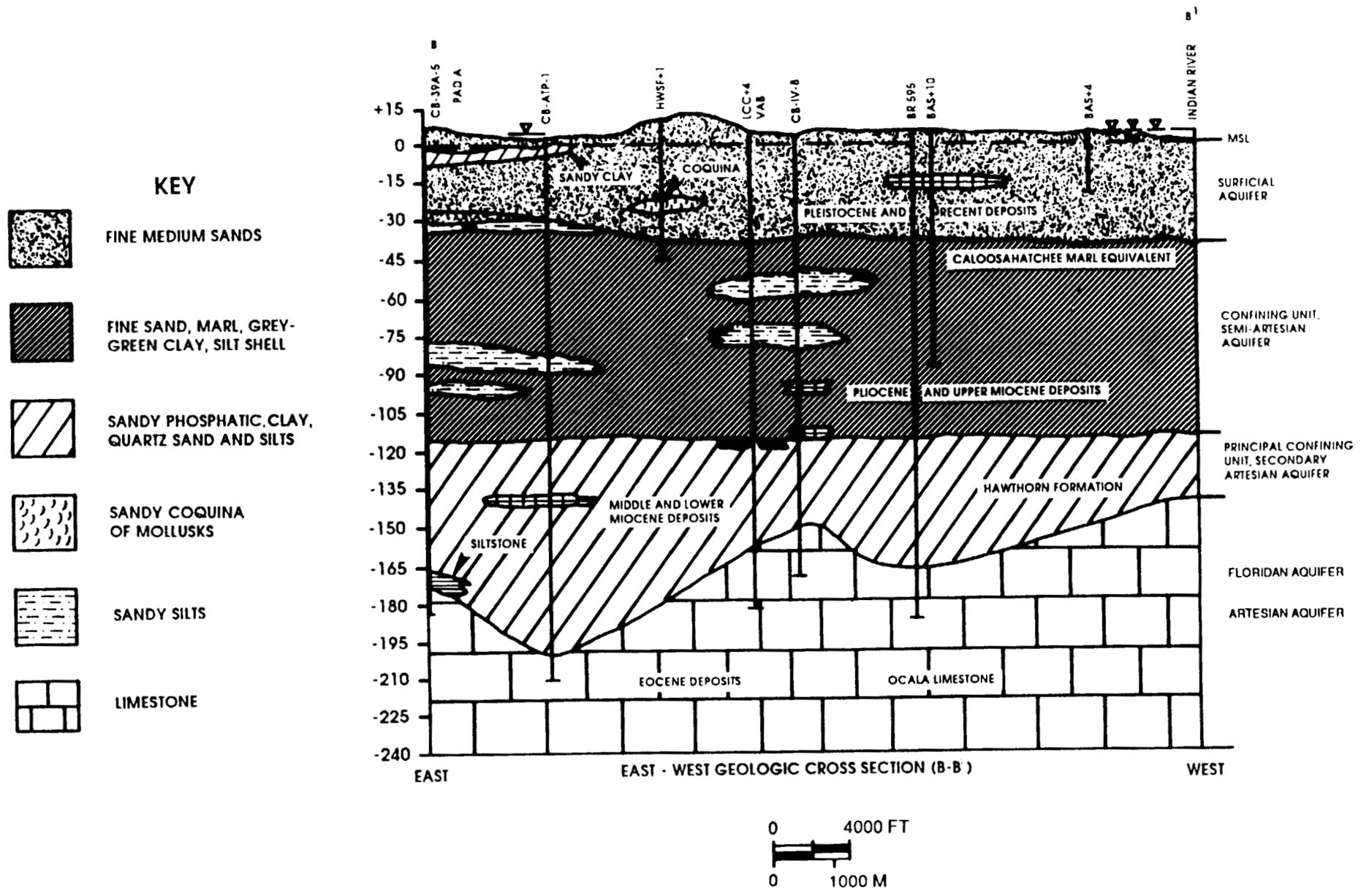
Figure 1.2. East-west geologic cross section, Kennedy Space center (redrafted from Clark 1987c). Vertical scale is elevation in feet relative to mean sea level.
