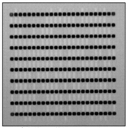
Optical image of inlet channel openings under bonded and lapped glass film. FIG. 13
