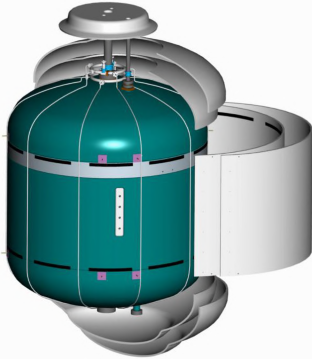
Figure 13.—Multilayer insulation (MLI) blanket configuration.
