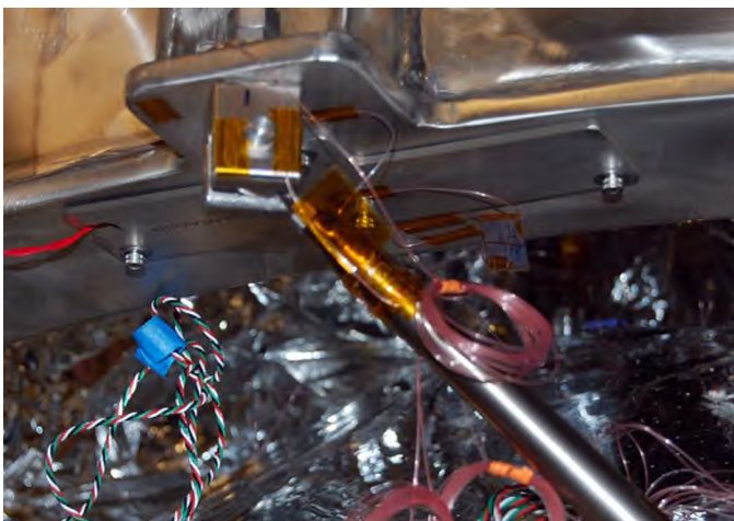
Figure 24.—Strut instrumentation and support ring heater.
