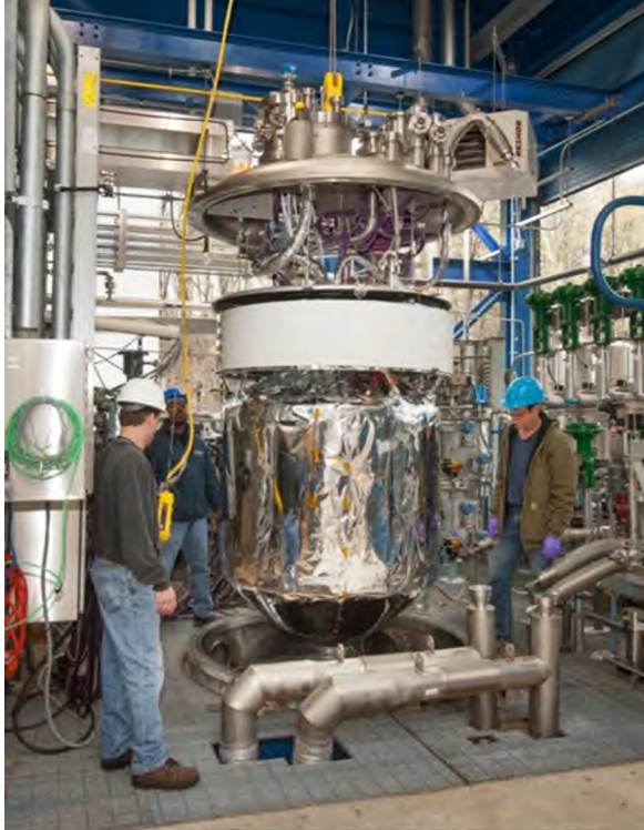
Figure 5.—Test article being lowered into the Small Multi-Purpose Research Facility (SMiRF) vacuum chamber.
