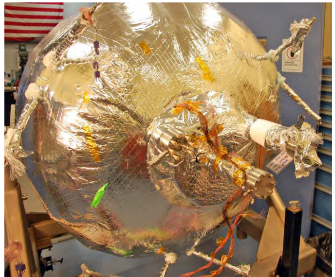
Figure 53.—Tank multilayer insulation (MLI) system prior to inspection.
