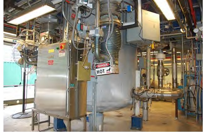
Figure 6.—Small Multi-Purpose Research Facility (SMiRF) vacuum chamber with diffusion pump and the Residual Gas Analyzer (RGA) in the foreground.
