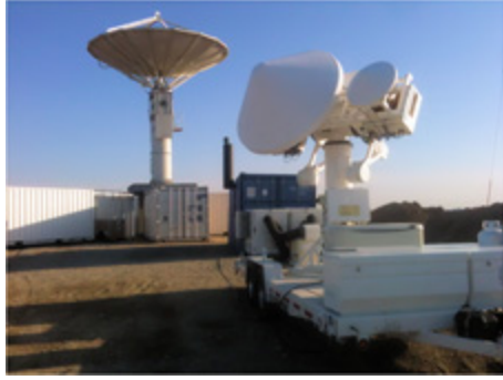
The NASA NPOL (left) and D3R (right) precipitation radars deployed south of Waterloo, Iowa, for the Iowa Flood Studies ground measurement campaign.
