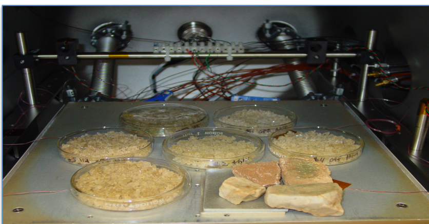
Figure 2. The salt crust in the Mars Simulation Chamber
