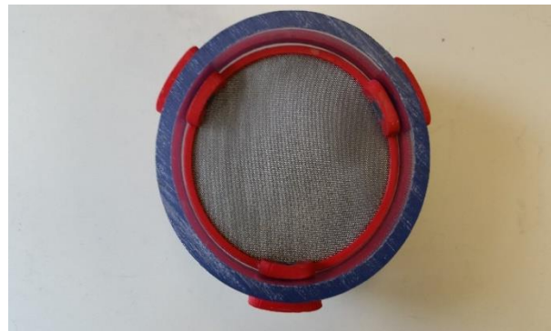
Figure 17b – Top view of magnetically-coupled, adjustable-height sand disperser.
