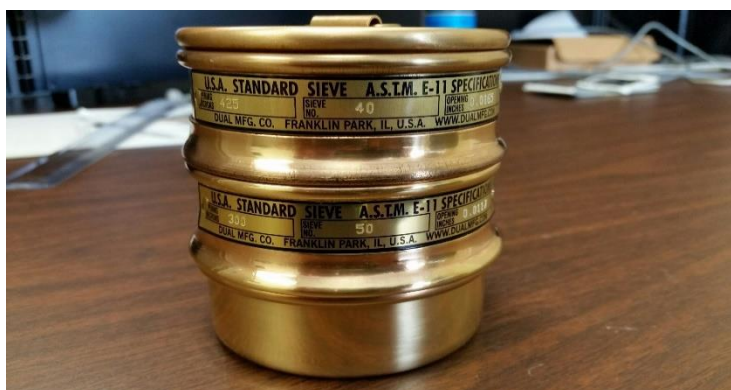
Figure 13 – 40 & 50 Standard Sieves used on particle sample sets.
