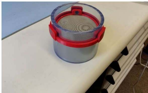
Figure 17a – Side view of magnetically-coupled, adjustable-height sand disperser.
