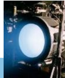
NEXT ion thruster demonstrates >51,000 hours of operation
